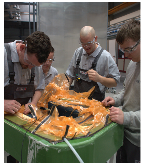
Application of webbed carbon
